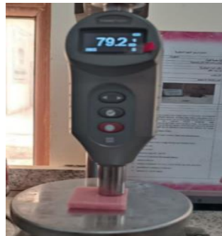
Figure 3: Device for measuring Shore D hardness
