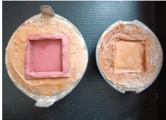
Figure 1: A silicone mold for surface hardness after the plastic designs have been invested and removed.
