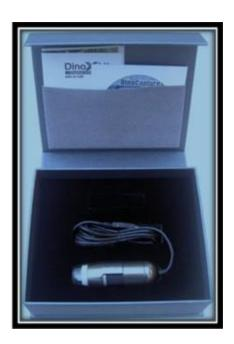
Each impression image's middle horizontal line was measured with a 300X zoom and a digital lens microscope with 0.001 mm accuracy (Soft Imaging System, 2013).
