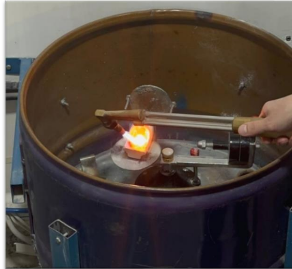
Figure 9: Heating of the metal using flame torch.
