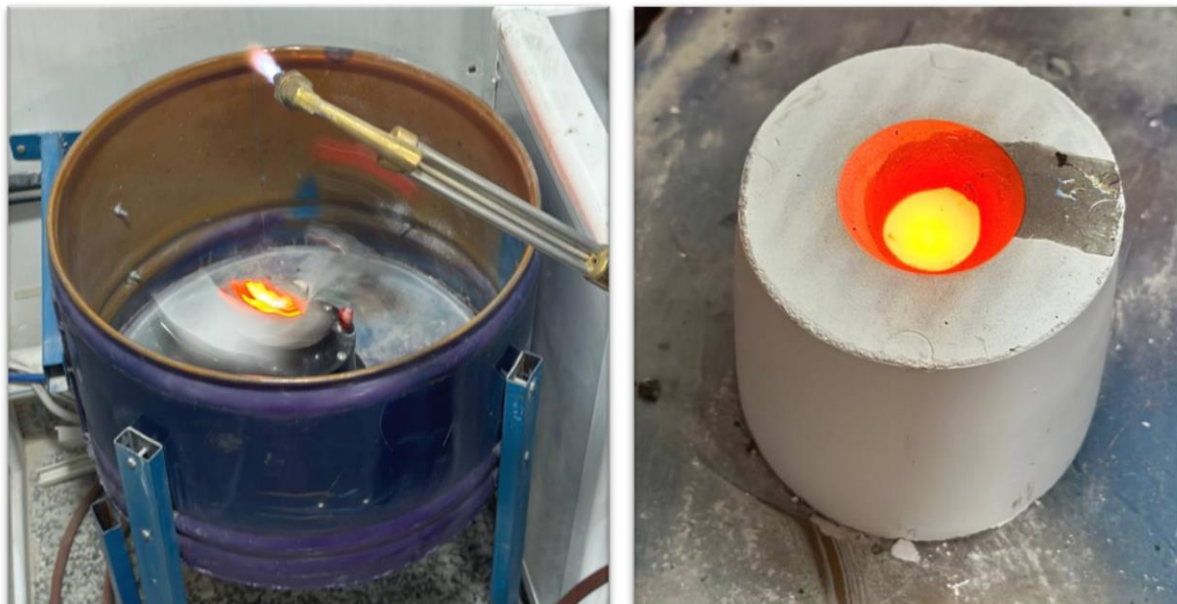
Figure 10: (A) Casting procedure, (B) Mold after casting procedure.
