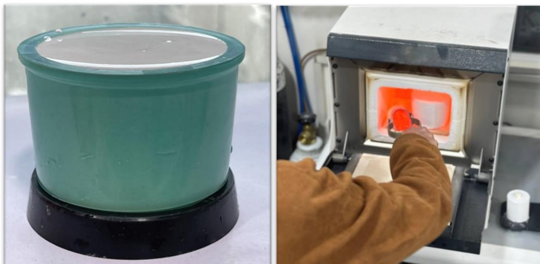
Figure 8: (A) Crucible former after pouring, (B) Mold in burnout furnace.
