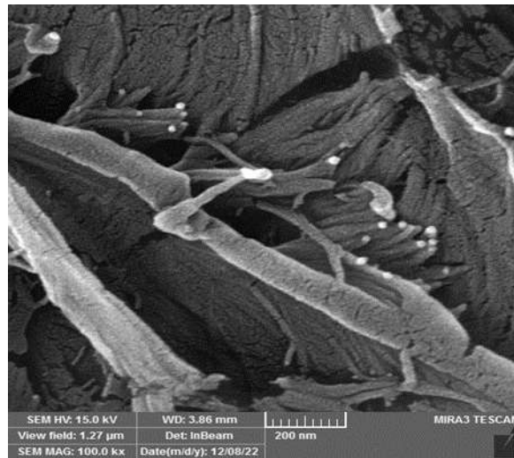
Figure (4): FESEM chitosan powder
