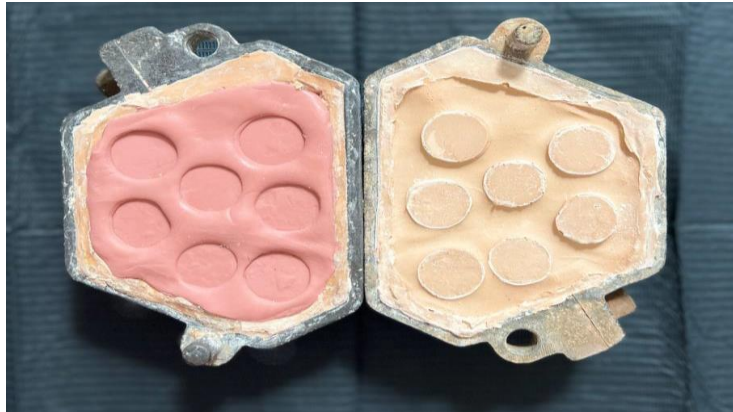
Figure 2: A silicone mold is utilized to evaluate the color permanence of a stone after its placement.
